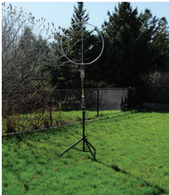
Figure 16 — The PWRC setup with a low-noise loop.
