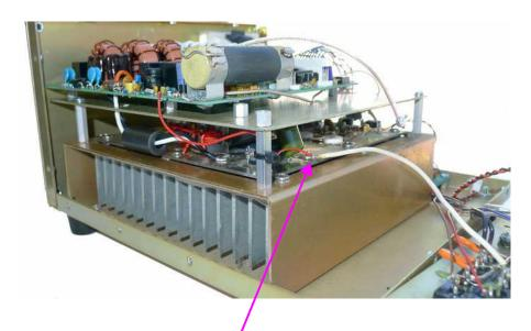
Solder red wire for 48VDC to PA module
