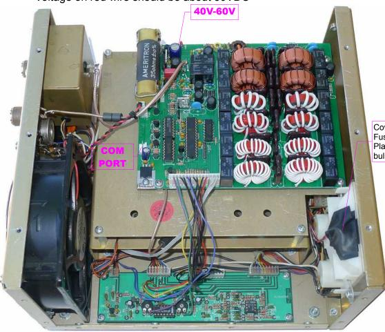
Cover can fall and short +12V Fuse inside PS will be blown! Place Electrical tape over bulb leads for protection.
